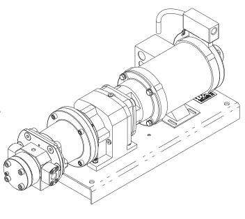
The 9000MD offers a static seal alternative to traditional mechanical and compression type dynamic seals. A permanent magnetic coupling transmits torque by magnetic forces between the internal and external rotors, through a statically sealed barrier. The barrier is constructed from stainless steel, nickel alloy or other corrosion resistant material and is not contacted by either the inner or outer rotor.
