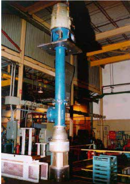
IMO 413IC-800JD pump mounted to the end of a discharge column. The drive shaft and spider bearings are inside the column.
