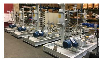
A PC pump consists of a rotor (or eccentric screw) surrounded by an elastomeric or metallic stator. Allweiler is one of the few global PC pump manufacturers to produce specially formulated elastomeric stators completely in-house to fit a wide range of applications. Quality control and testing for the stators is performed in-house by Allweiler, at the highest standards.
