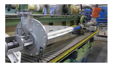
PC pump materials are particularly suitable for highly contaminated or high BS&W fluids such as produced water and raw gas condensates and can accommodate fluctuating working pressure, low NPSH and variable fluid viscosities with ease.
