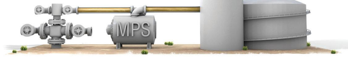
MP 250 has helped to increase the production rate by providing the energy to overcome the pressure differential between the wellhead and the separator.
